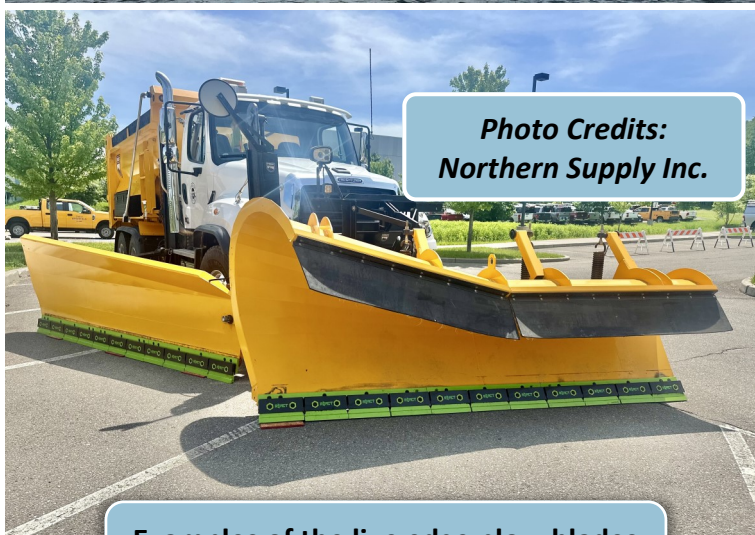
Examples of the live edge plow blades which will help reduce road salt usage
